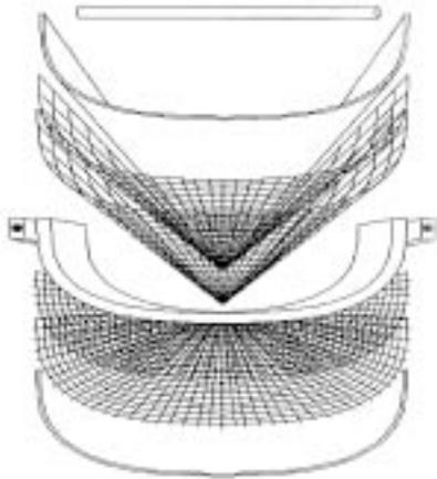
Fig. 1: 3-D exploded view of the reinforced concrete composite section of the hull skin
