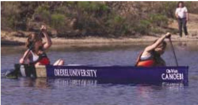
Fig. 5: The final product included several layers of water sealant, automotive primer, paint and clearcoat, and stenciled vinyl lettering (photo courtesy of ASCE/MBT)
