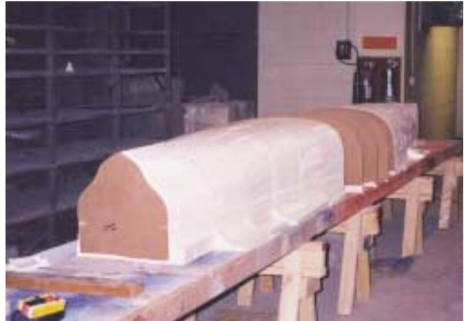
Fig. 2: Mold composed of cross-sectional templates and EPS block mounted on a wooden strongback
