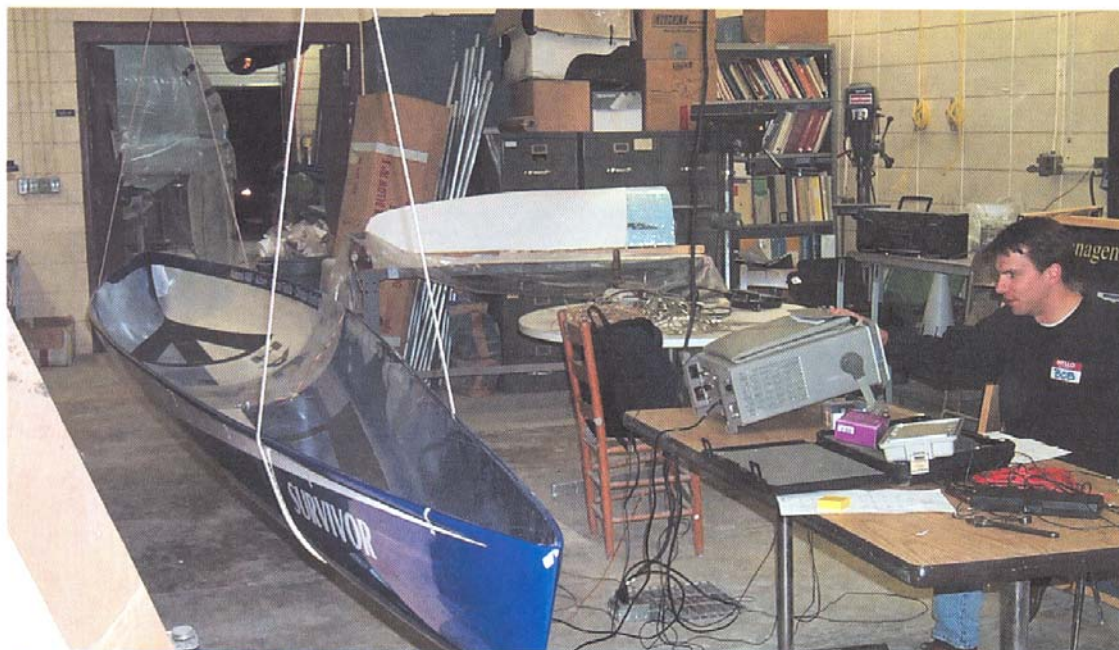
Figure 1. Survivor was tested in a free-hanging configuration
